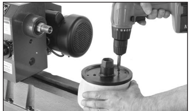
Figure 37. Typical attachment of faceplate to workpiece.
